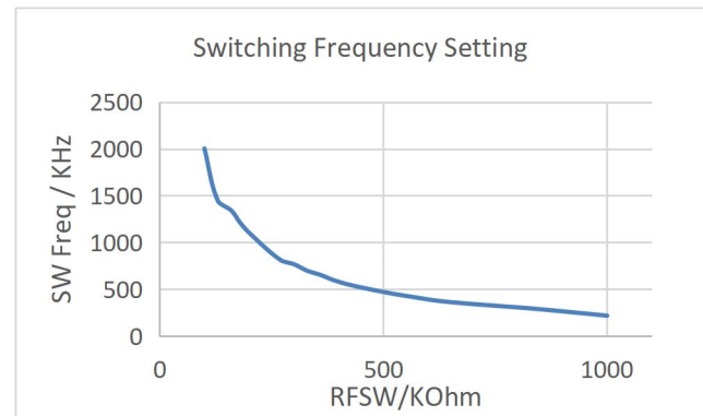
Figure 2 Switching Frequency Setting
