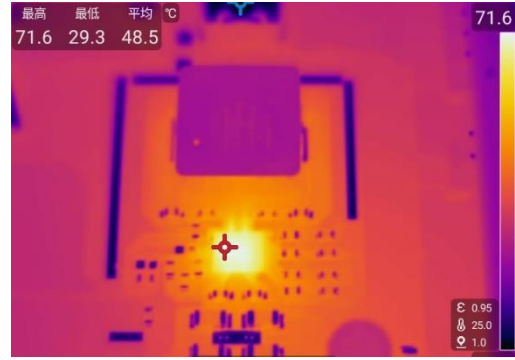
Figure 8-58. Thermal Image; V_{IN}=12V , V_{OUT}=20V , I_{OUT}=3.25A , f_{SW}=420kHz , top/bottom layer: 2oz, mid-layer: 1oz, disable external switch Q1
