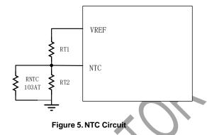
Use below equations to calculate the RT1/RT2 resistance when a 103AT NTC thermistor is used as shown in Figure 5.
